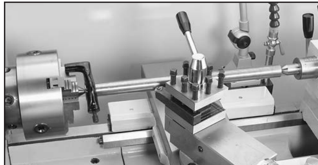
Figure 43. Example photo of a workpiece mounted between two centers.
